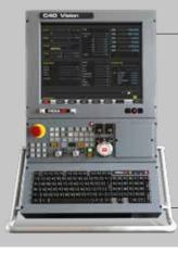
The C40 Vision numerical control is an innovative solution for machining in a modern and efficient way. By integrating the software ViMill® offers performance and features of highest level and extraordinarily effective for the control and the safety of machine tools.
