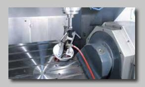
Upper gantry structure with high rigidity monolithic basement and integrated roto-tilting table.
