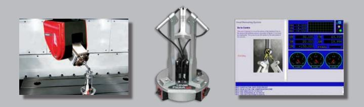
The HMS system is a device designed to check and correct geometric errors of continuous and indexed bi-rotary heads as well as roto-tilting tables.
