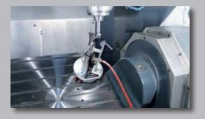
Upper gantry structure with high rigidity monolithic basement and integrated roto-tilting table. Ideal for high precision 5 sides and 5 axis machining. The machine is fully equipped with active thermal control.
