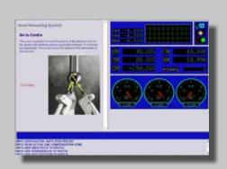
The HMS system is a device designed to check and correct geometric errors of continuous and indexed bi-rotary heads as well as roto-tilting tables.
