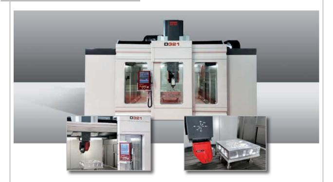
D321 has a compact size with a very large working envelope designed for mold finishing applications. The wide opening front door is ideal for loading large and heavy workpieces while offering an unsurpassed visibility. Fast and precise, D321 take advantage of specific FIDIA head choice, continuous or bi-indexed, according to the application.
