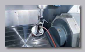
Upper gantry structure with high rigidity monolithic basement and integrated roto-tilting table. Ideal for high precision 5 sides and 5 axis machining.
