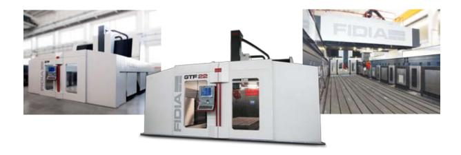
The new GTF Gantry machine Line, identified by a wide operative volume modularity, combines High Speed performances with great structural stiffness.
