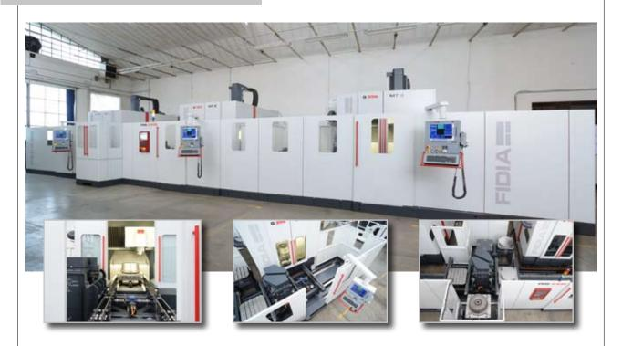
The platform integrates a pallet system shared by two or more machines. A powerful dedicated software, automatically manages and optimizes the flow of production without intervention of the machine operator. Each machine can be also used in a standalone way, nonetheless granting the normal functioning of the FMS system with the other machines.
